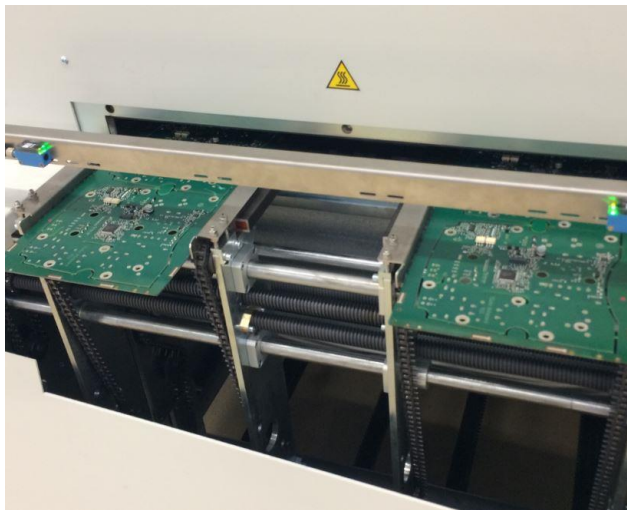
Figure 19. Boards parallel loaded with the same conveyor speed.
