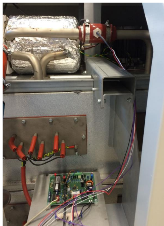
Figure 4. The lambda sensor mounted after the catalyst. The sensor is installed in the last peak zone. To protect the lambda sensor a catalyst is placed in front of the sensor. Both sensor and catalyst are placed outside the zone. Due
