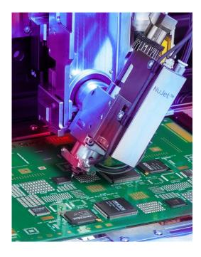
Setup and calibration are automated functions that run after the machine has been initialized and/or if the pump has been removed and replaced. These routines ensure that the camera needle off sets at different angles and rotations are known.
