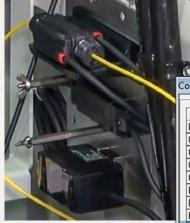
The flux flow monitor sends alarms if flow rate is out of tolerance, flux line leak is detected, flux volume is out of tolerance, or fluxer flow is restricted.
