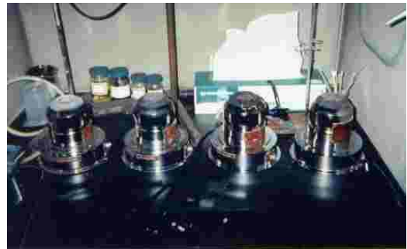
Figure 3 – Solder Exposure Baths
