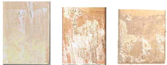
Figure 9 Uncoated 316 SST Samples Wetting present on all samples.
