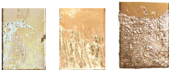
Figure 7 Uncoated 304 Stainless Steel Samples Wetting Present on all samples.
