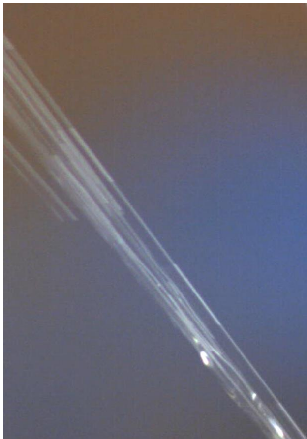
Figure 16. The spray bundle of the drop jet.
