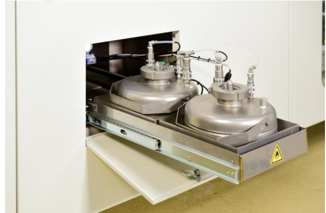
Figure 1. The main flux vessel is refilled by the flux from the replenish tank during production.
