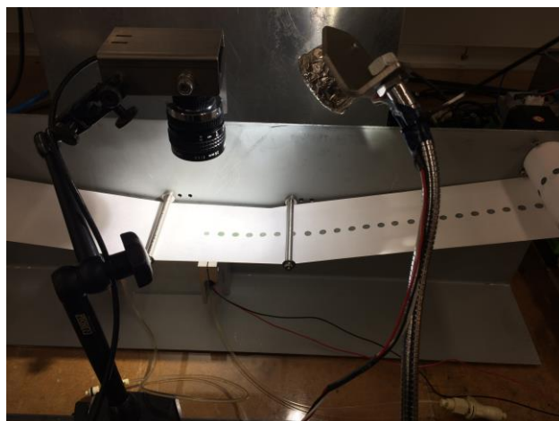
Figure 17. Test setup with drop jet spraying on paper and camera measuring the position and shape of the droplet.
