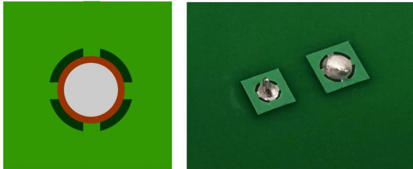
**Figure 9: Thermal relief and solder mask**
