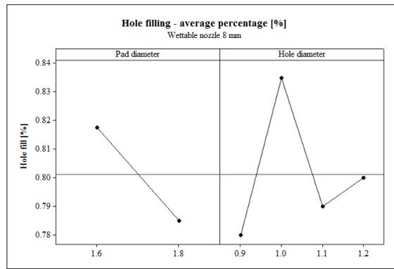
**Figure 6: Hole filling [%] for an 8 mm wettable nozzle.**
