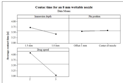
**Figure 5: Factorial Plot of 8 mm wettable nozzle, showing the effect of parameters on contact time.**
