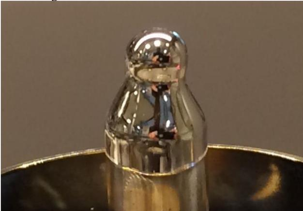
**Figure 3.** A bullet type nozzle made of wettable material.
