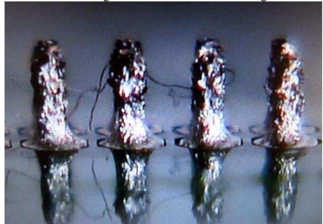
**Figure 18:** Fine pitch component showing hairline bridges after soldering.
