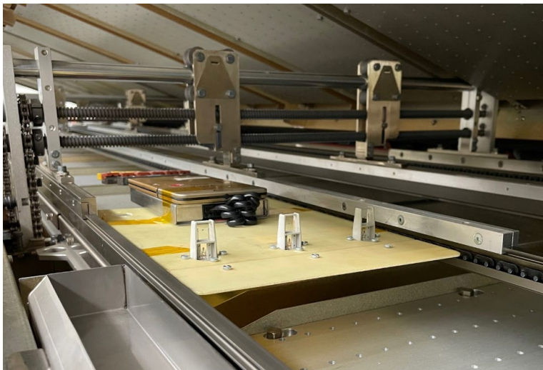
77 Figure 2. Three Probes Measuring the Horizontal Gas Flow During Transportation Through the Reflow 78 Oven. 79
