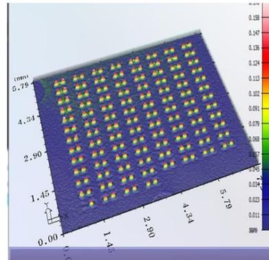
Figure 8: Overview of paste deposits 008004'' (0201mm)
